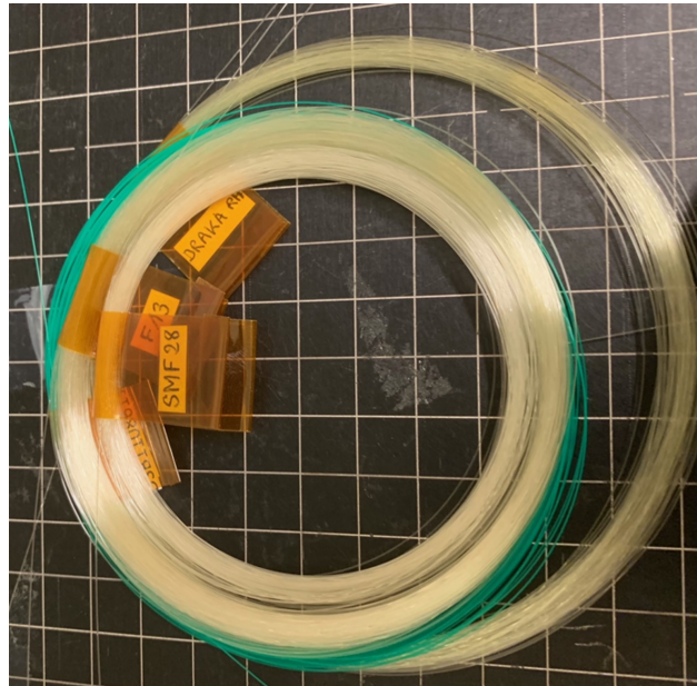
Figure 3.7: Example of the optical fibers that were characterized to be used within the DOFRS system.
