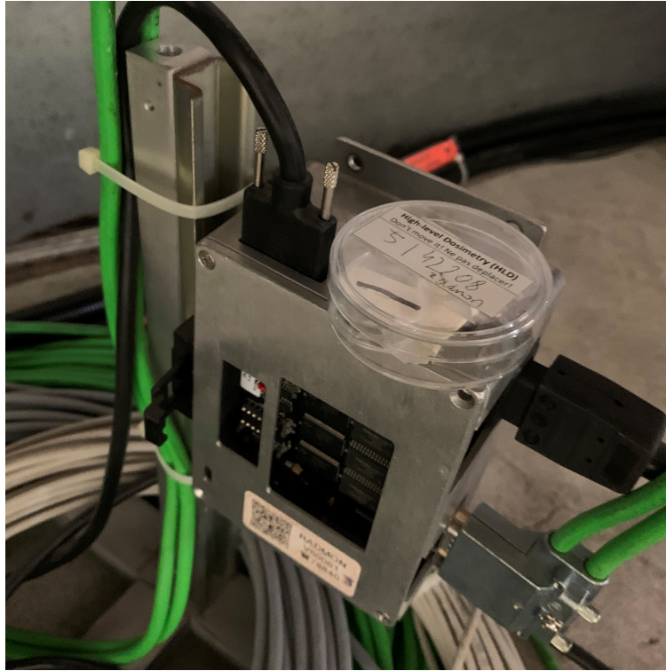
Figure 3.9: RadMon with RPLd installed in the SPS.
