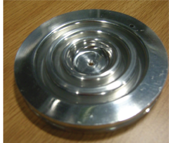
Figure 1: A two-choked 8 GHz Al test cavity.
