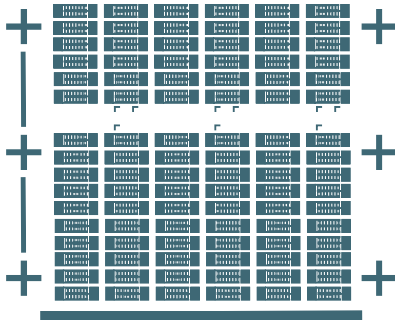
Fig. 4.13 Lithography mask design for e-actuated trumpets.
