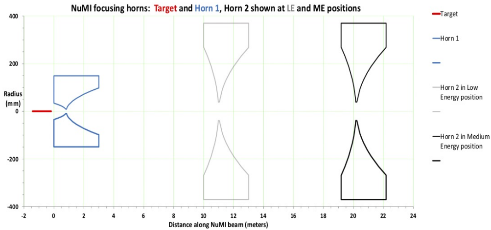
Figure 4.4: The NuMI target fins (red) as seen from above with the two focusing horns. Horn1 (blue) starts at MCZERO. Horn2 is shown in ME (black) and LE (gray) positions. Note that the vertical axis is in millimeters, while the horizontal axis is in meters.
