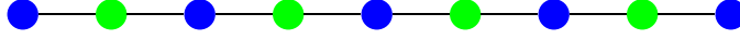
Figure D1. A one-dimensional cluster state with nine vertices as the B_c subgraph.
