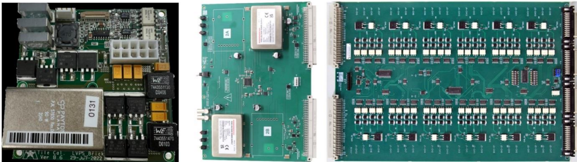
Figure 4: Low voltage brick (left). High voltage supply board (center) and HVremote board used for the individual regulation of the voltage for 48 PMTs (right).
