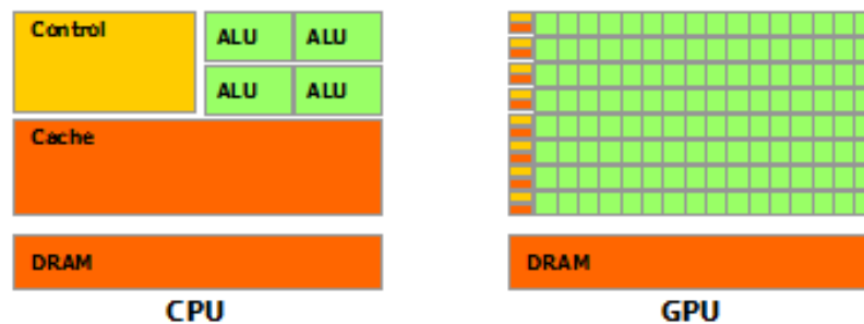
Figure 1-6. GPU devotes more transistors to data processing (ALU)[49].
