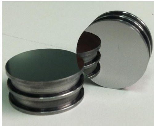
Figure 3-6. Photograph of polished molybdenum pucks before deposition of the photoemission layer.
