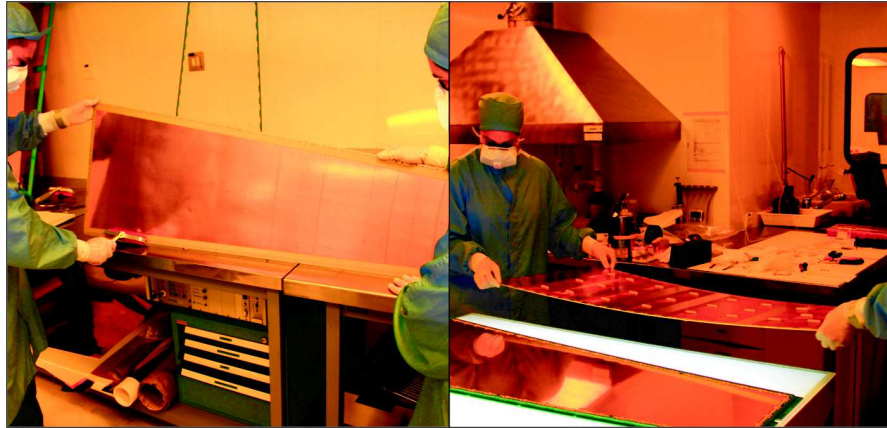
FIGURE B.15: Step 15: after being cleaned (left), the readout board is placed on top of the external frame to close the chamber.
