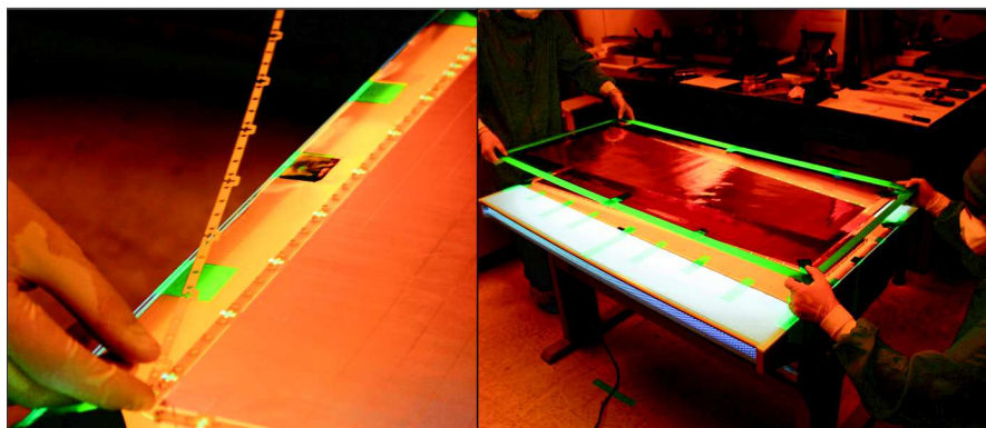
FIGURE B.5: Step 5: the second layer of internal frames is placed on top of the first GEM (left). After testing and cleaning, the second GEM is added to the stack (right).
