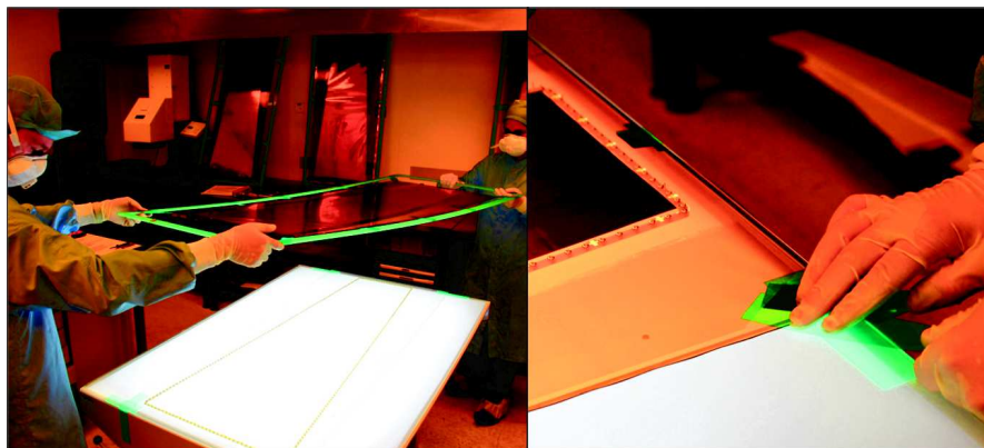
FIGURE B.4: Step 4: the first GEM is placed on the first layer of internal frames (left). The foils is stretched by hand and attached to the working table to ensure the flatness and stability of the structure (right).
