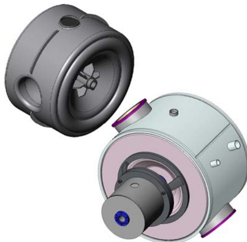
Fig.2. HINS cavity and cavity / helium vessel / solenoid assembly.
