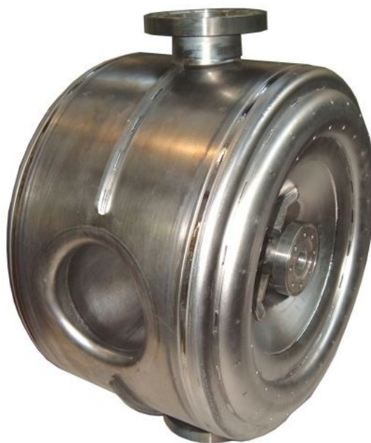
Fig. 9. One of the first two spoke resonators delivered from industry and the first test article for this cryostat.
