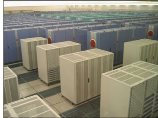
(2002) Earth Simulator: 640 nodes, 35.8 TFLOPS
