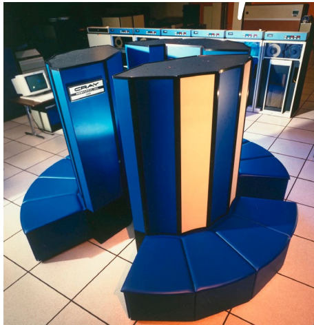
(1985) Cray-2 Supercomputer: 250 MHz cpu, 1.9 GFLOPS
