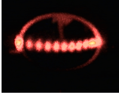
Figure 3.7: Image showing multiple reflections between two reflecting surfaces as in an MPLC system. This image was captured in the summer of 2016 when I did a research internship in the Lundeen group. The mirror-mirror separation is 10 cm and ten reflections are achieved on a mirror of diameter 2.54 cm. I used a webcam for taking this image, the webcam introduced visual distortion probably due to an ultra wide-angle lens. Mirror appears ellipsoidal rather than circular, and spots appear circular when they were produced to be elliptical by using cylindrical lenses. Reflections do not lie on a straight line due to the use of a cylindrical mirror for implementing this MPLC. Notice that subsequent results used a new implementation of the MPLC as described in Section 3.3.
