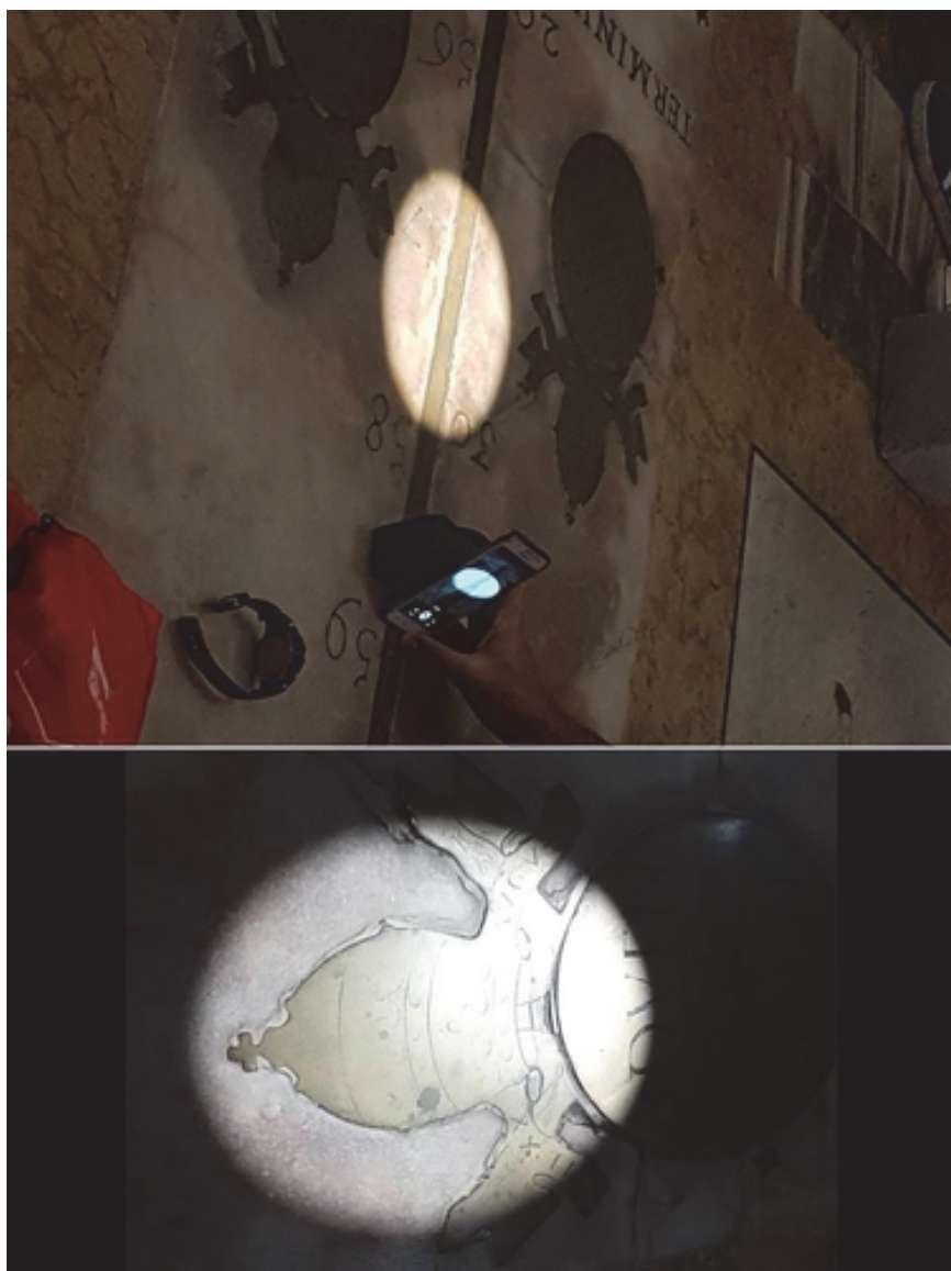
Fig. 2. The Sun on the XX August MDCCII inscription, on 21 August 2019. Its penumbra is 38.6% of the pinhole width, instead of 100% geometrical. Air humidity 55%.
