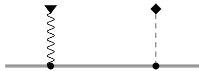
Figure 1. Feynman diagram corresponding to the leading order contribution of new physics to the g factor of a bound electron. The double line represents the bound electron, the wavy line terminated by a triangle represents interaction with an external magnetic field, and the dashed line terminated by a rhombus denotes the electron–nucleus interaction via exchange by a scalar boson.
