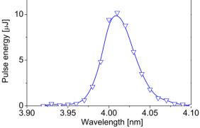
Figure 3: Frequency doubler at FLASH2 (experimental data). Left: gain curve of the frequency doubler at FLASH 2. First part of the undulator (5 modules) is tuned to 8 nm, and second part (7 modules) is tuned to 4 nm. Red and blue color correspond to the radiation wavelength of 8 nm and 4 nm. Right: radiation pulse energy at the 2nd harmonic versus resonance frequency of the second part of the undulator. Electron energy is 1080 MeV, bunch charge is 300 pC.
