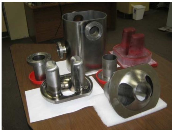
Figure 57: Niobium parts of UK 4-Rod Cavity [21]. Figure 58: Photo of UK 4-Rod Cavity [20].
