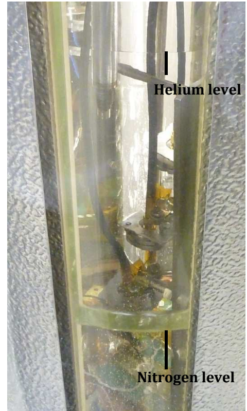
Figure 51: Setup in the glass cryostat. At the top one can slightly see the helium level and much lower the nitrogen level.
