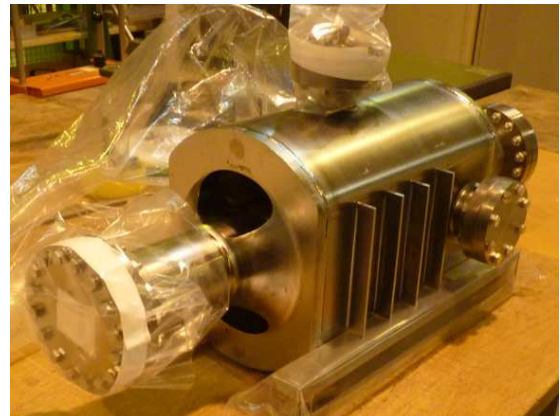
Figure 57: Niobium parts of UK 4-Rod Cavity [21]. Figure 58: Photo of UK 4-Rod Cavity [20].
