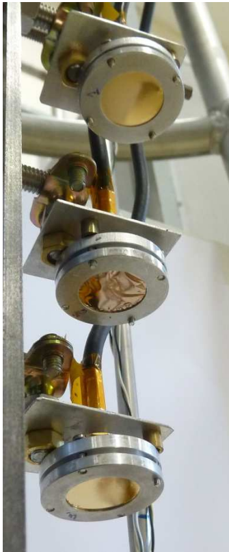
Figure 53: Photo of the three OST membranes in the test setup at room temperature.
