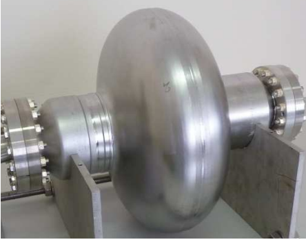
Figure 2: Photo of an elliptical one-cell cavity (for SPL).
