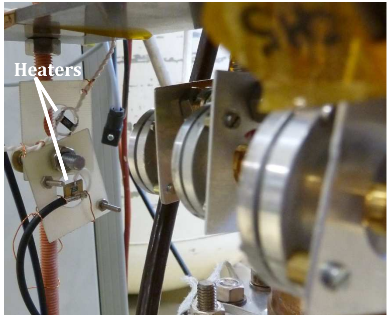
Figure 42: Photo looking along the three OSTs on the heaters (DC top, RF bottom).
