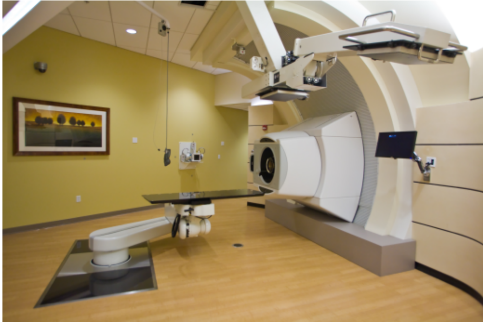
Figure 1.12: One of the patient rooms prior to the setup of the PPS test bench, on the right side of the picture the snout of the proton delivery system is visible and the robotic table is in the center
