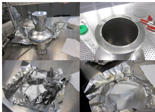
Figure 3: C3C4 after the coating run. Note discoloration on the NbTi cavity flange (top right) and 'tin' droplets on the niobium foil from the cavity top flange.
