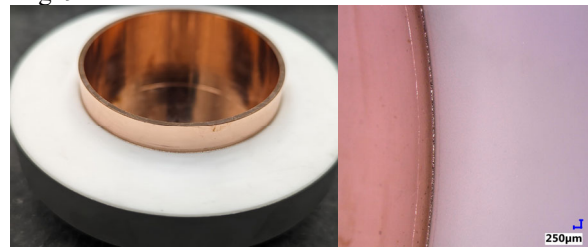
Figure 8: (Left) Second ID test braze assembly showing clean joint without excess alloy flow. (Right) close up view of braze joint.
