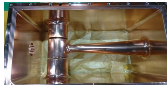
Figure 4: Buncher main body after first machining and Assembled cavity inner dimension.
