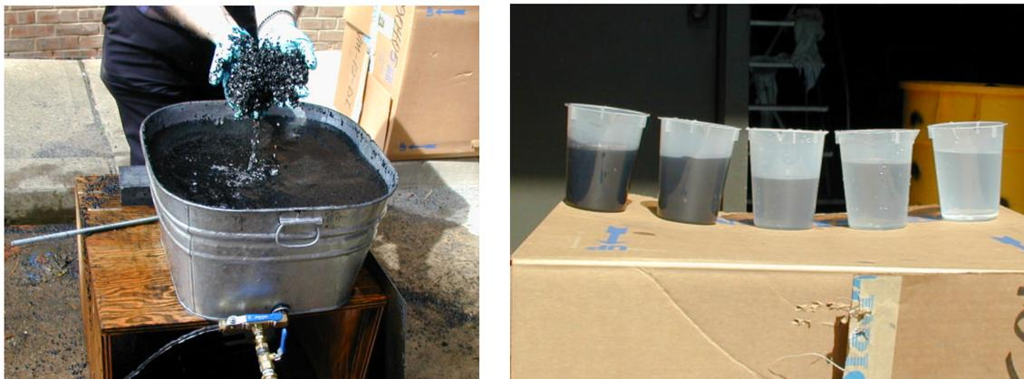
Figure 5.3: Washing the activated charcoal for the radon filter (left). The rinse water was monitored until the visible level of dust was negligible (right).
