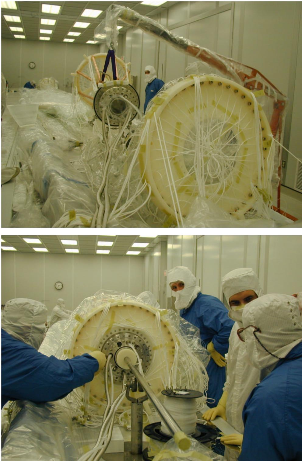
Figure 6.11: Nesting the IV inside the OV. The north pole IV assembly is bolted to the OV end region. The load cell bellow conduits and the two spools for the IV and OV optical fibers can be seen in the foreground (bottom).
