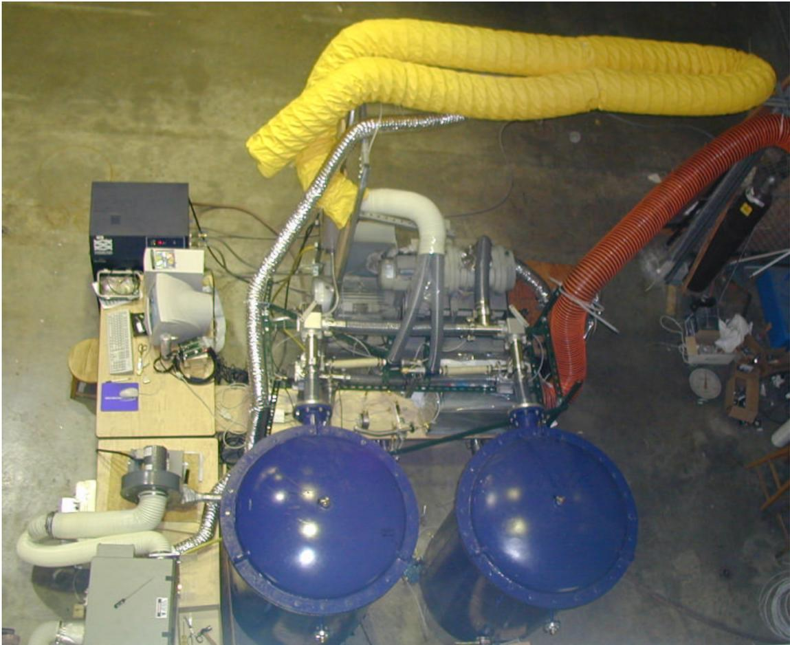
Figure 5.5: Top view of the charcoal-based VSA radon filter for the Borexino vessel construction clean room. On the left, from the bottom, are the silica gel drier, the input air blower, the control computer, and the chiller for the roots blower. The big hose at the top of the picture serves as a muffler for the re-pressurization air intake, otherwise very noisy. The connection to the clean room is via the hose on the right.
