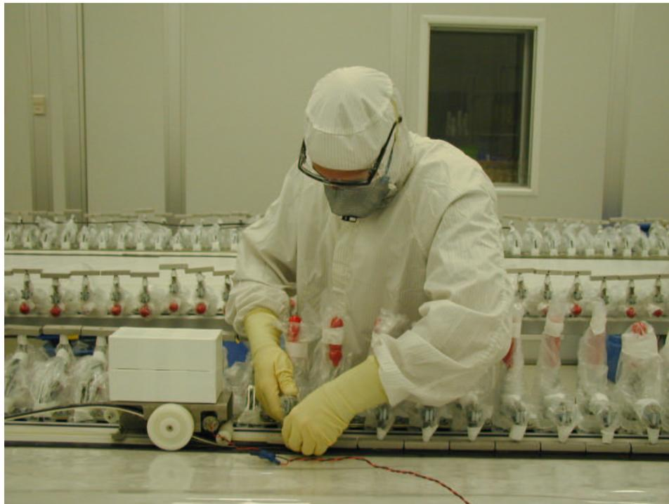
Figure 6.6: Closing the clamps on a vessel glue joint for mechanical strength and leak tightness of the seal.
