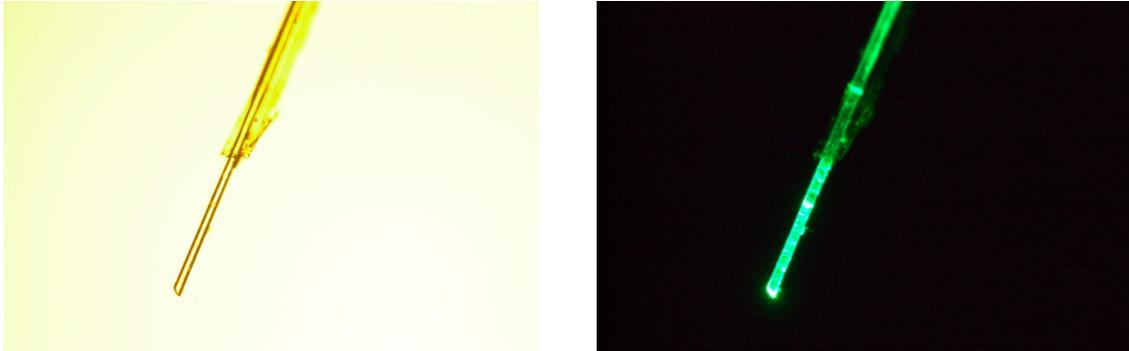
Figure 7.1: Optical fiber tip etched in hydrofluoric acid in ambient light (left) and illuminated with a green laser light (right). Significant amounts of light could be scattered away from the forward direction by removing the polyamide coating wrapping around the quartz core. Because of the low reproducibility of the results, fragility of such fibers and the complications related to using aggressive chemicals in the clean room environment, the design was abandoned.
