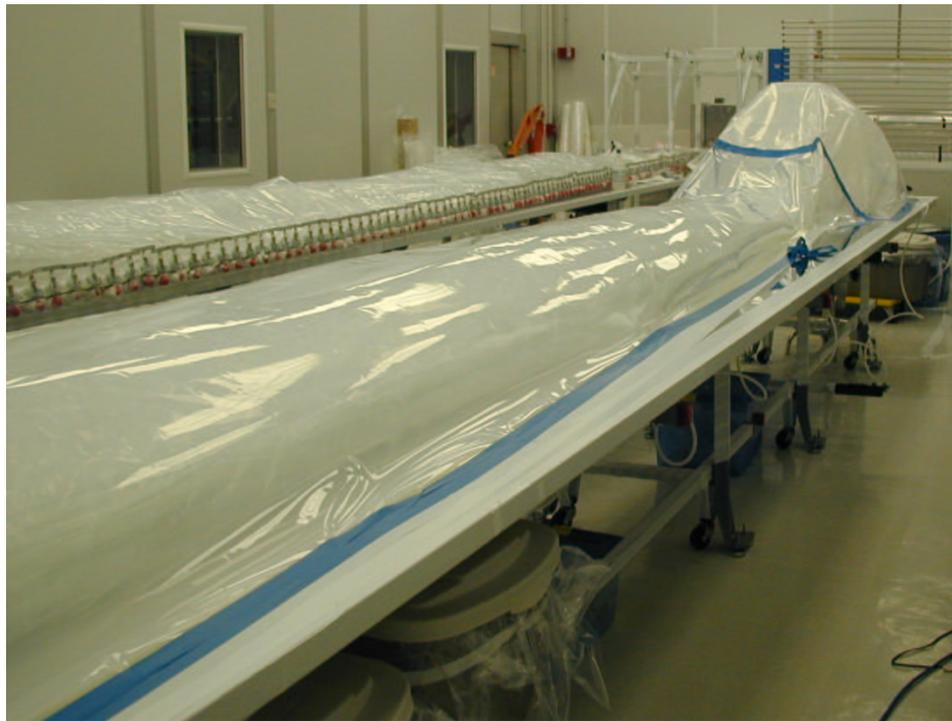
Figure 6.18: The sealed Borexino IV is filled with  $\text{SF}_6$  for leak checking. A bag is placed around it to collect  $\text{SF}_6$  leaking out. After an adequate accumulation time is allowed to pass, the accumulation bag is opened up and the  $\text{SF}_6$  concentration inside the clean room is measured, giving the integrated leak rate.
