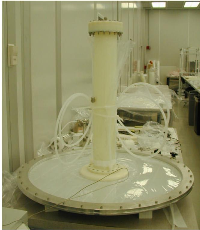
Figure 6.17: One IV nylon pipe + bridge film assembly assembled and prepared before being glued into the vessel. The assembly is mounted on a device that allows leak checking with  $\text{SF}_6$  gas. The two  $3/8$ " flexible nylon sampling lines are also mounted at this stage. The capillary tube from the mass spectrometer used to sniff for  $\text{SF}_6$  is also visible.
