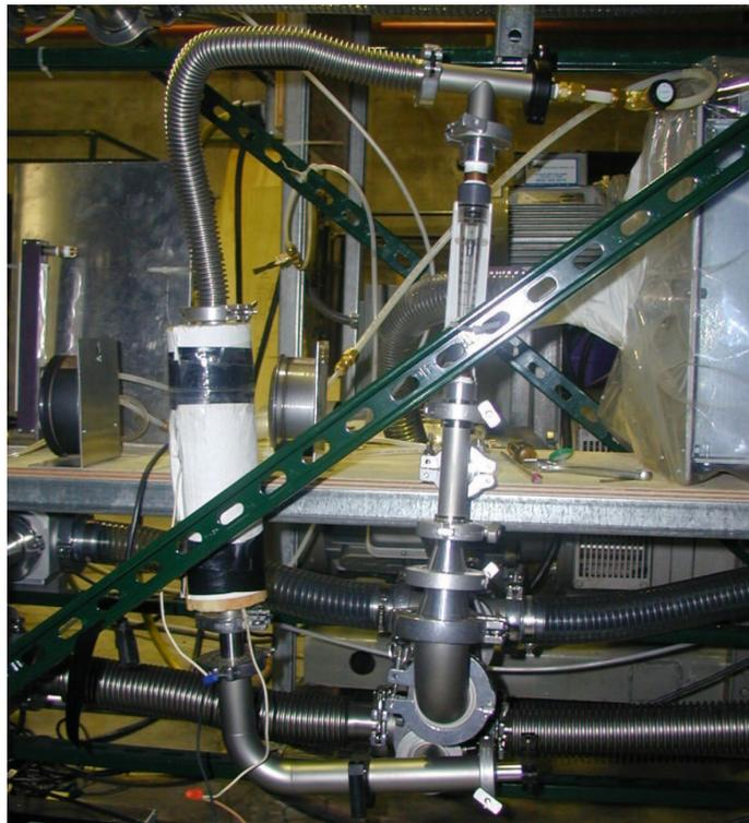
Figure 5.7: Closeup of the purge regulating line.
