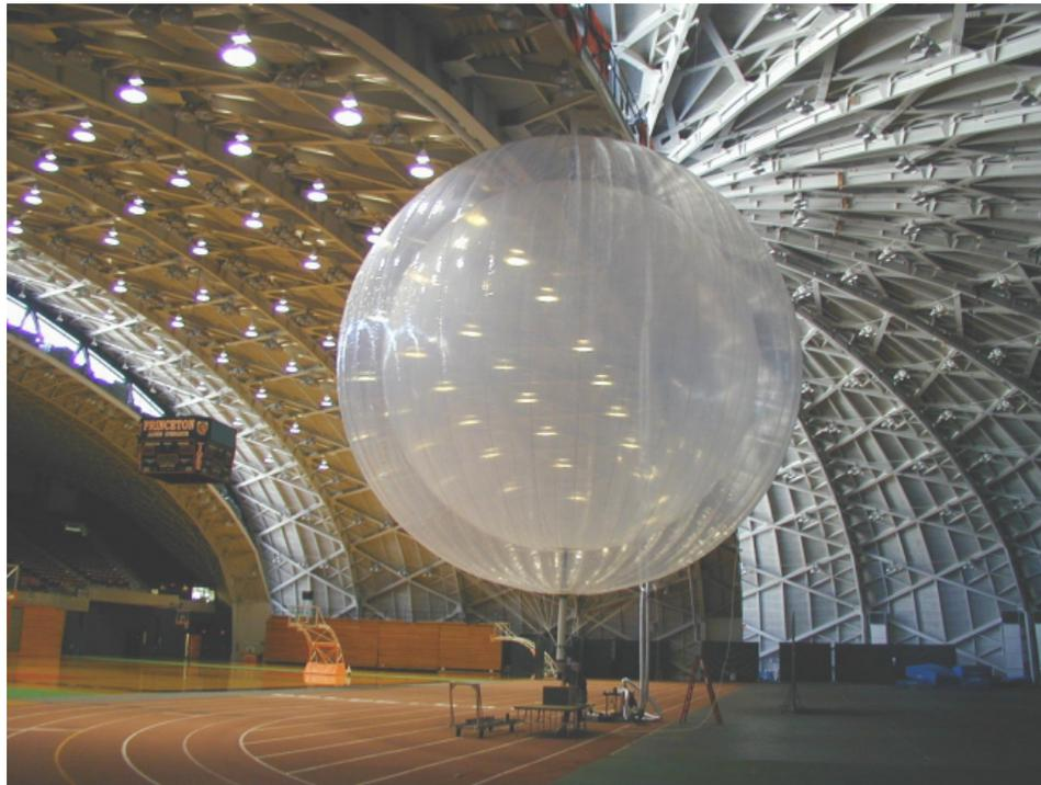
Figure 3.2: Full scale prototypes of the Borexino Inner Vessel (top) and Inner+Outer Vessels nested set (bottom). The two vessels are respectively 8.5 and 11 m in diameter, and were inflated inside Princeton's indoor gymnasium, the only building on campus able to accommodate their size when inflated. The diameter of the final Borexino OV is 11.5 m.
