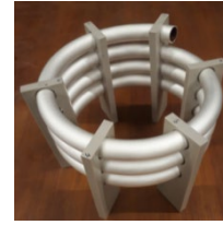
Figure 6: Coil made from standard copper plumbing, silver coated.
