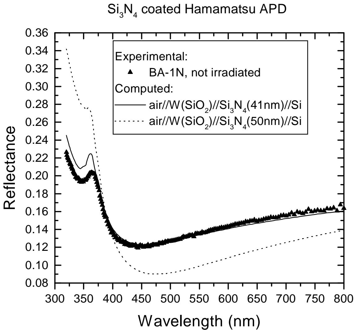
**Fig. 7:** reflectance of the  $\text{Si}_3\text{N}_4$  coated “BA1N” Hamamatsu APD compared with the computed reflectance based on the model “air//W( $\text{SiO}_2$ )// $\text{Si}_3\text{N}_4$ (41nm)//Si”. The effect of the  $\text{Si}_3\text{N}_4$  antireflection coating is more effective in the 400-520 nm range when the coating thickness is about 50 nm.
