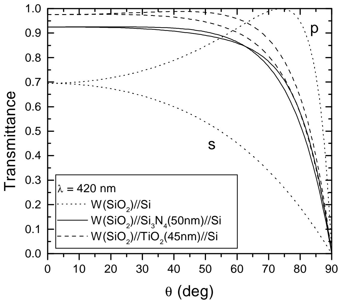
**Fig. 8b:** transmittance at 420 nm versus the incidence angle from  $\text{W}(\text{SiO}_2)$  to the Si without and with  $\text{Si}_3\text{N}_4$  (50nm) and  $\text{TiO}_2$  (45nm) AR.
