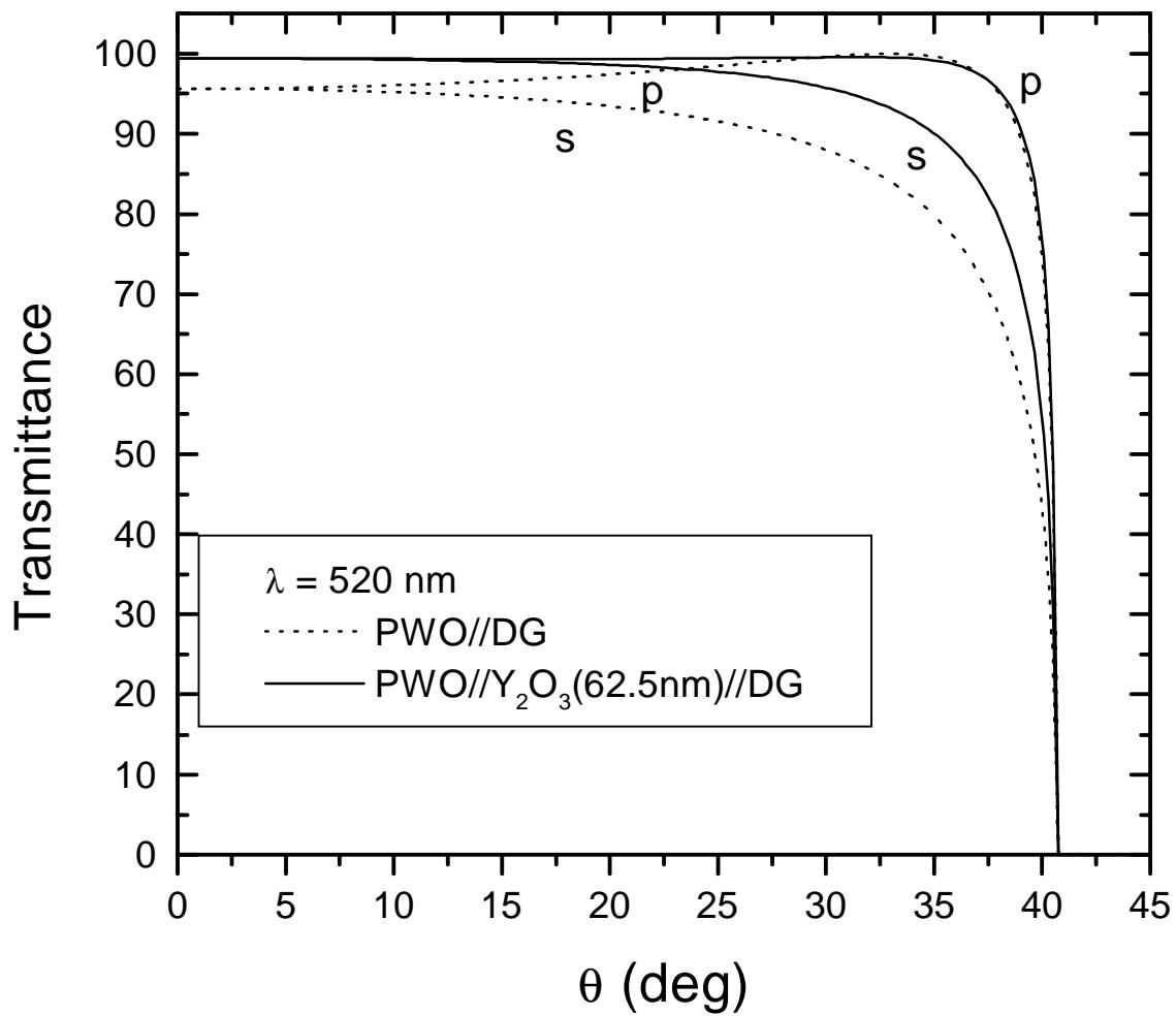
**Fig. 13b:** simulated transmittance versus incidence angle at 520nm of the interfaces PWO//DG and PWO// $\text{Y}_2\text{O}_3(62.5\text{nm})$ //DG.
