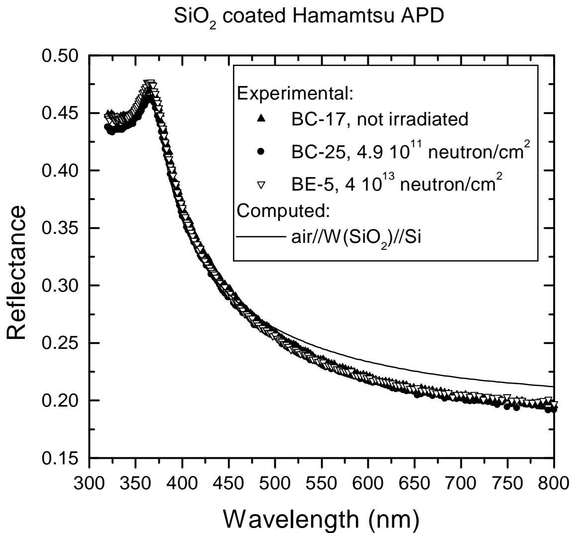
**Fig. 6:** reflectance of BC-17, BC-25 and BE-5 Hamamatsu APD, irradiated with neutrons at several doses compared with the reflectance computed according to the model “air//W//Si”, where the refractive index of the rubber window (W) is assumed to be the same of the  $\text{SiO}_2$  coating.
