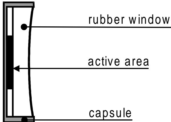
**Fig. 1:** section of APD's produced by EG&G and Hamamatsu. In both devices the Si wafer is enclosed in a capsule and covered with a transparent window. In the EG&G APD (Fig. 1a) the window is sealed to the capsule with some transparent glue. The Hamamatsu (Fig.1b) adopts a rubber window which completely fills the capsule-room and cover the Si surface together with the electric contacts (not reported in the figure).
