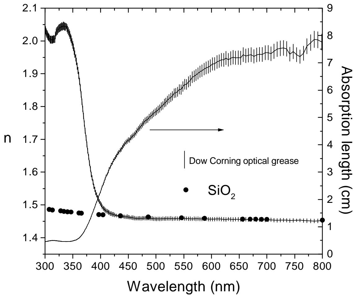
**Fig. 9:** measured refractive index and absorption length of the Dow Corning 02-3067 optical grease. For wavelengths greater than 400nm the refractive index is very similar to the  $\text{SiO}_2$  (fused silica) one, also reported in figure [5].
