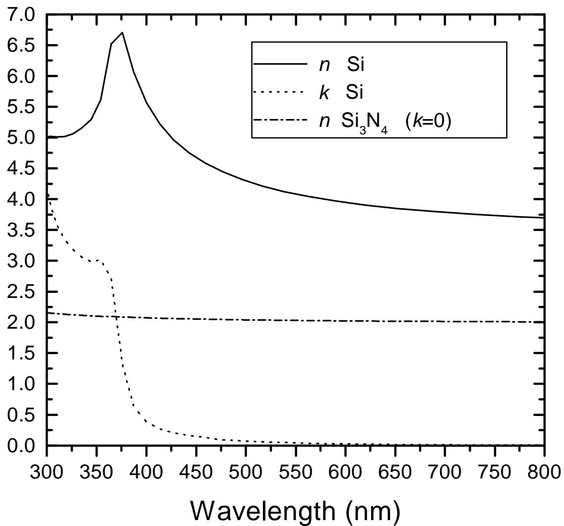
**Fig. 5a:** complex refractive indexes of Si and  $\text{Si}_3\text{N}_4$  [5].
