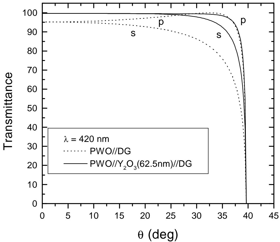
**Fig. 13a:** simulated transmittance versus the incidence angle at 420nm of the interfaces PWO//DG and PWO// $\text{Y}_2\text{O}_3(62.5\text{nm})$ //DG.
