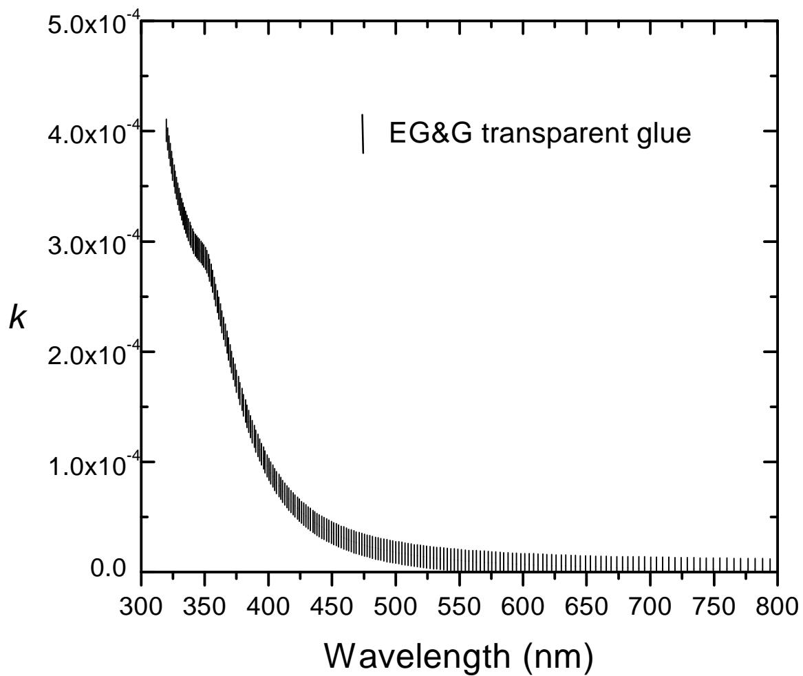
**Fig 5b:** extinction coefficient of the  $30\mu\text{m}$  thick transparent glue (TG) layer, placed between window and Si in the EG&G APD, giving a good reproduction of the experimental reflectance measurement.
