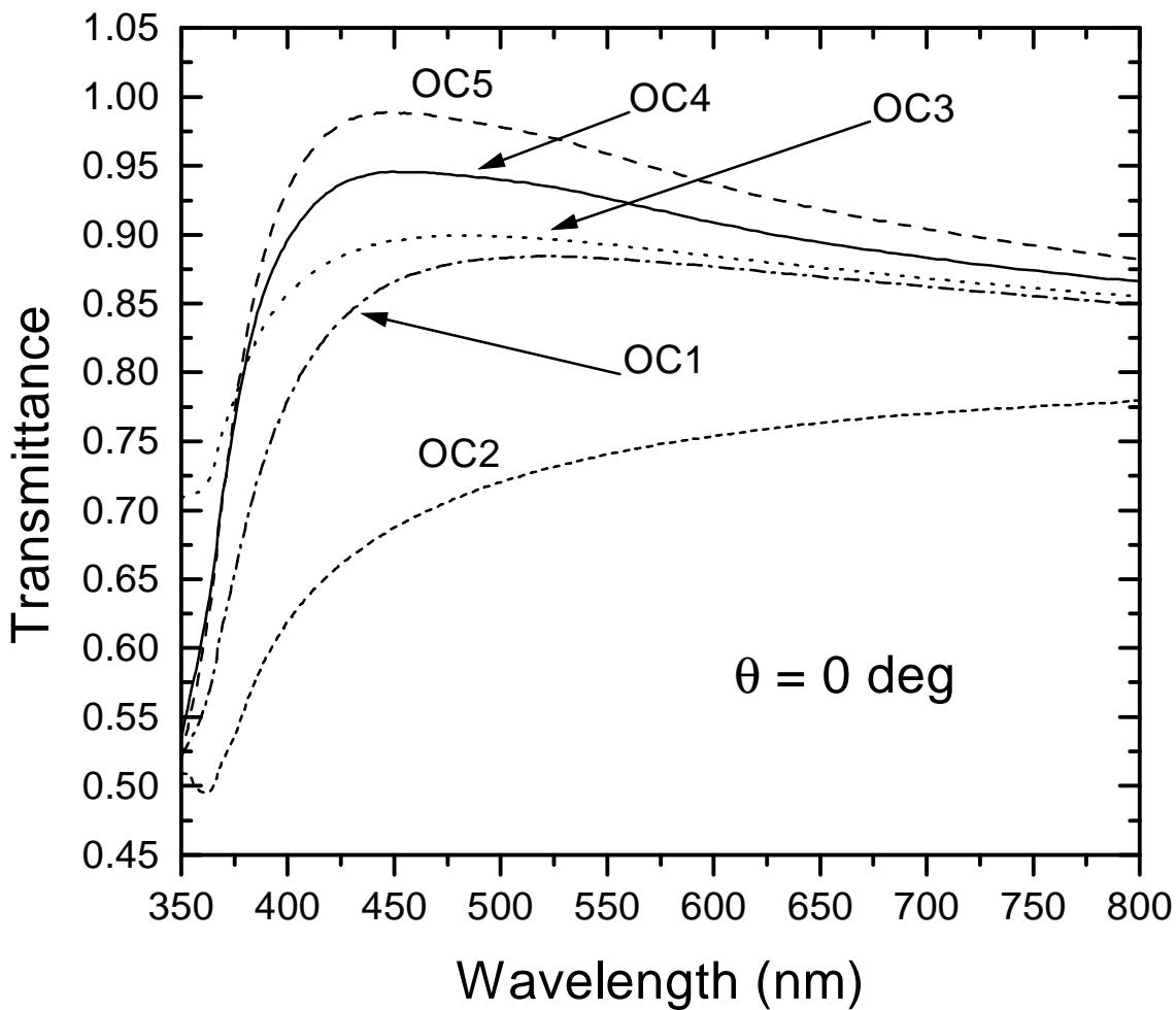
**Fig. 14a:** computed transmittance, from the PWO to the Si, at normal incidence for:
