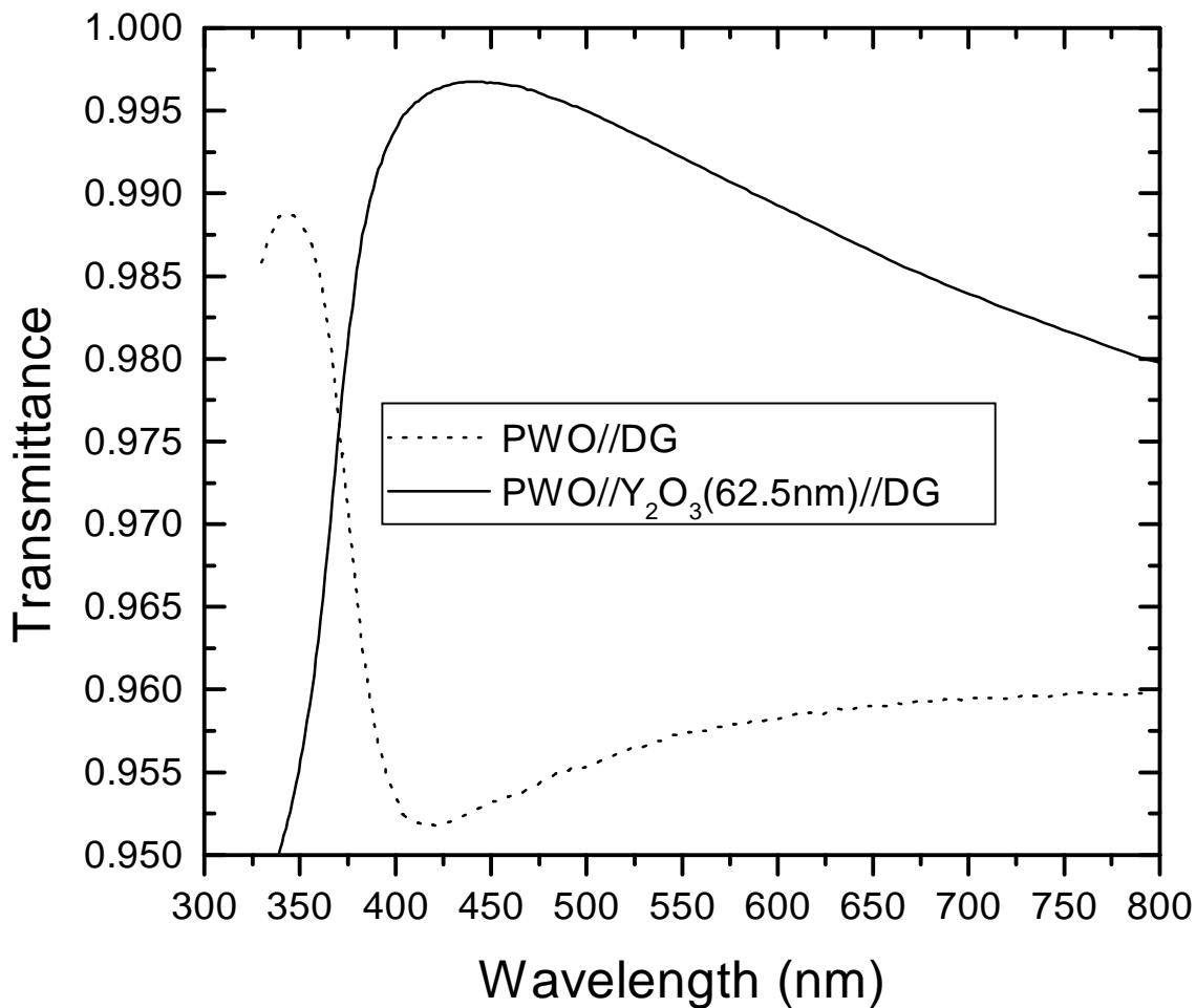
**Fig. 12:** simulated transmittance, at normal incidence, of the interfaces PWO//DG and PWO// $\text{Y}_2\text{O}_3(62.5\text{nm})$ //DG. With the AR coating the transmittance is about 4% greater than the uncoated case.
