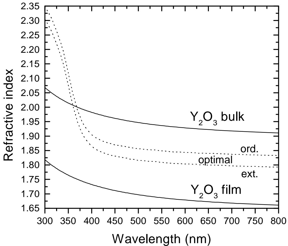
**Fig. 10:** refractive indexes of: a) the optimal AR coating for the PWO//DG interface ( $\sqrt{n_{PWO}n_{DG}}$ ), both for the ordinary and the extraordinary PWO refractive indexes; b)  $Y_2O_3$  bulk [7]; c)  $Y_2O_3$  film deposited on the PWO test piece as computed from the measurements reported in Fig. 11.
