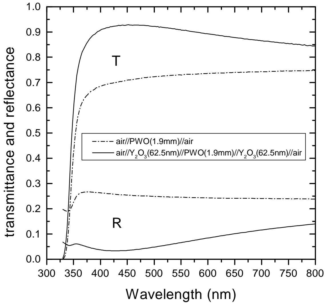
**Fig. 11:** transmittance and reflectance, at normal incidence, of the uncoated and coated PWO test piece. The experimental curves are well reproduced by assuming the films perfectly transparent ( $k=0$ ), 62.5 nm thick and with the refractive index of a material composed by 76% in volume of  $\text{Y}_2\text{O}_3$  [7] and 24% of air, computed according to the effective medium approximation [9].
