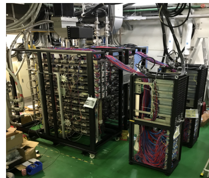
Figure 2: The 80kW solid-state amplifier with two separate power supply racks.
