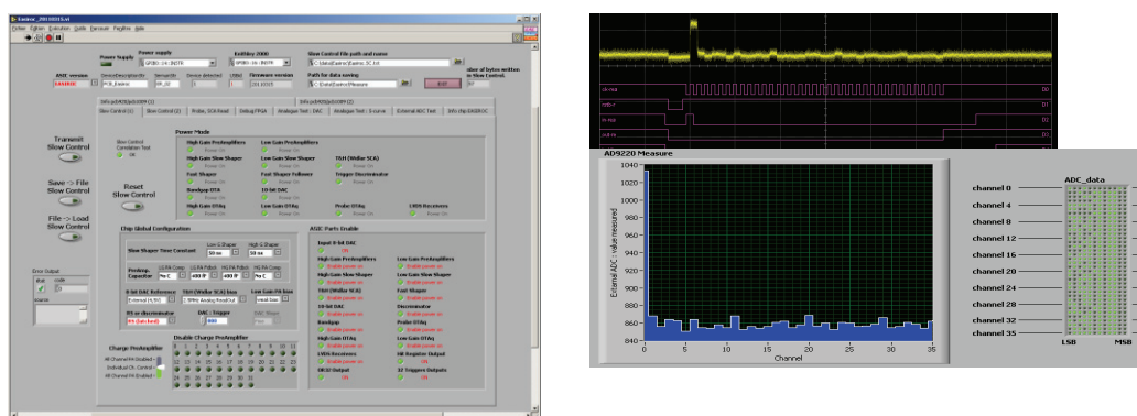
Fig. 10. EASIROC software (slow control and DAQ)
