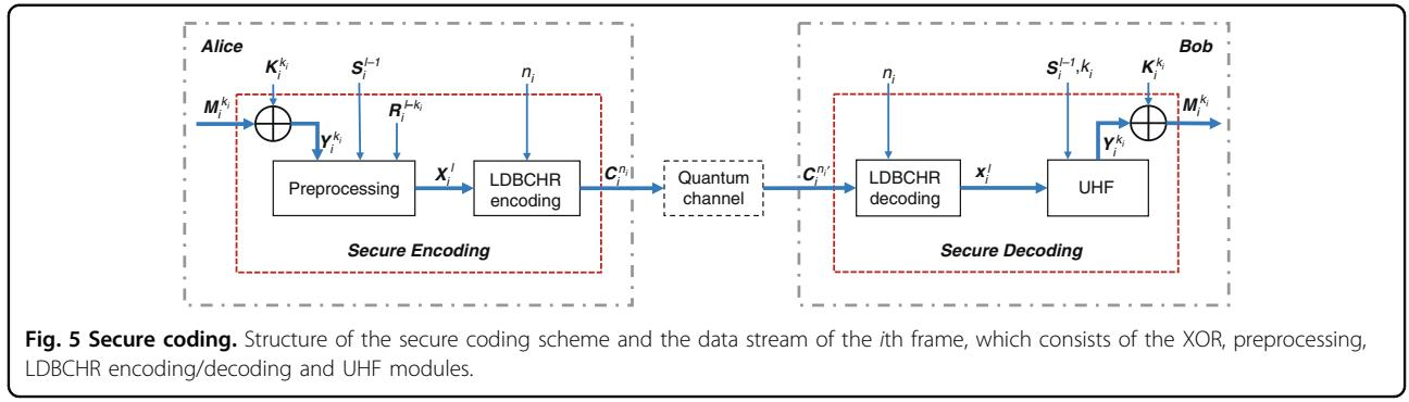
**Fig. 5 Secure coding.** Structure of the secure coding scheme and the data stream of the  $i$ th frame, which consists of the XOR, preprocessing, LDBCHR encoding/decoding and UHF modules.
