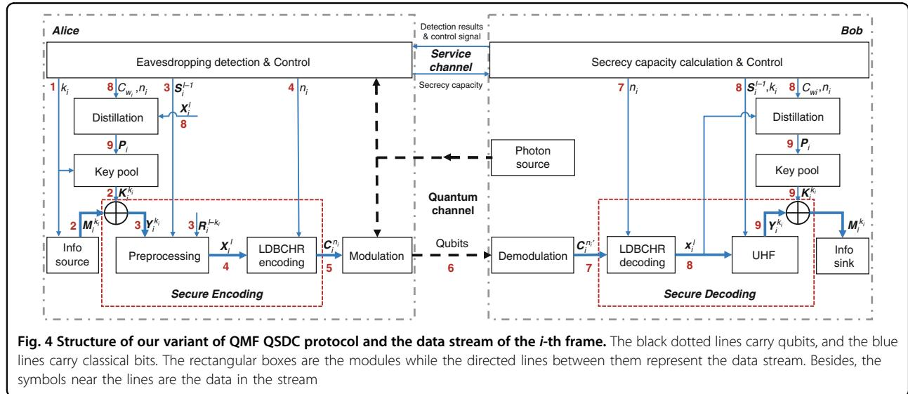
**Fig. 4 Structure of our variant of QMF QSDC protocol and the data stream of the  $i$ -th frame.** The black dotted lines carry qubits, and the blue lines carry classical bits. The rectangular boxes are the modules while the directed lines between them represent the data stream. Besides, the symbols near the lines are the data in the stream
