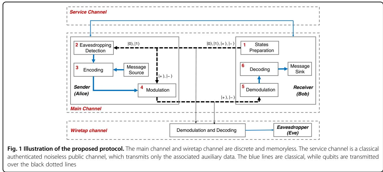
**Fig. 1 Illustration of the proposed protocol.** The main channel and wiretap channel are discrete and memoryless. The service channel is a classical authenticated noiseless public channel, which transmits only the associated auxiliary data. The blue lines are classical, while qubits are transmitted over the black dotted lines
