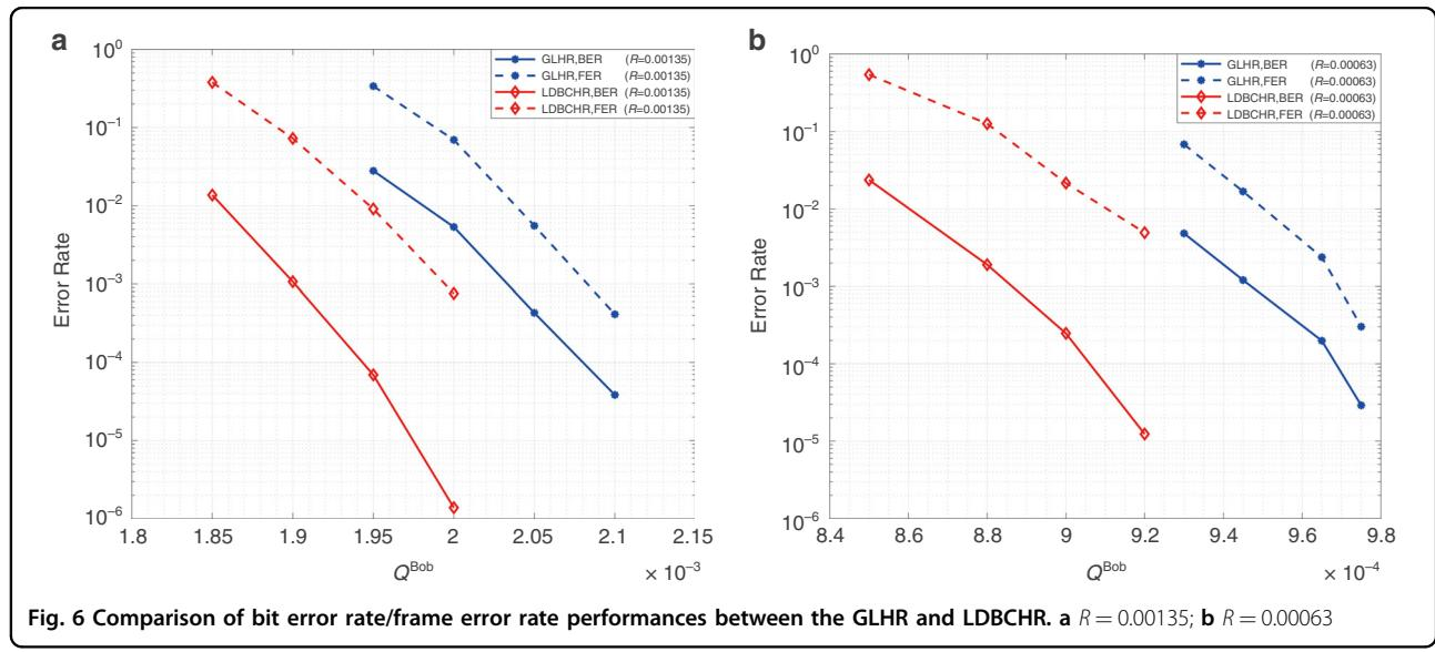
Fig. 6 Comparison of bit error rate/frame error rate performances between the GLHR and LDBCHR. a  $R = 0.00135$ ; b  $R = 0.00063$
