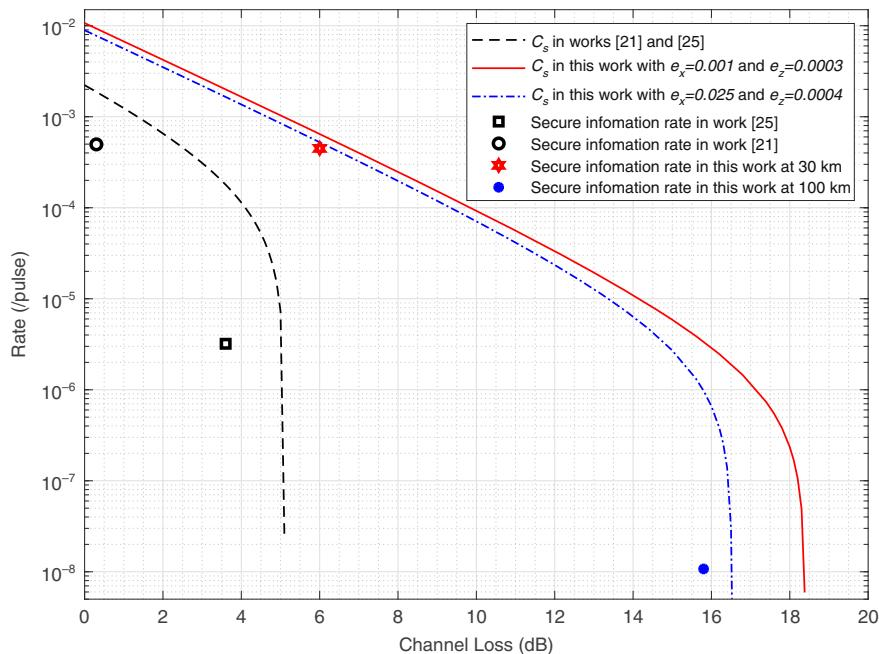
**Fig. 3** Simulation with experimental parameters. Comparison of secrecy capacity and secure information rate between previous works and this work.
