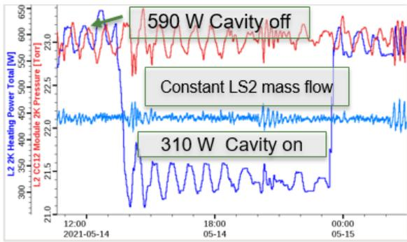
Figure 10: ARR05 run with LS2 at 2 K. Red: 2 K header pressure. Blue: total electrical heater power. Cyan: mass flow of 2 K system.
