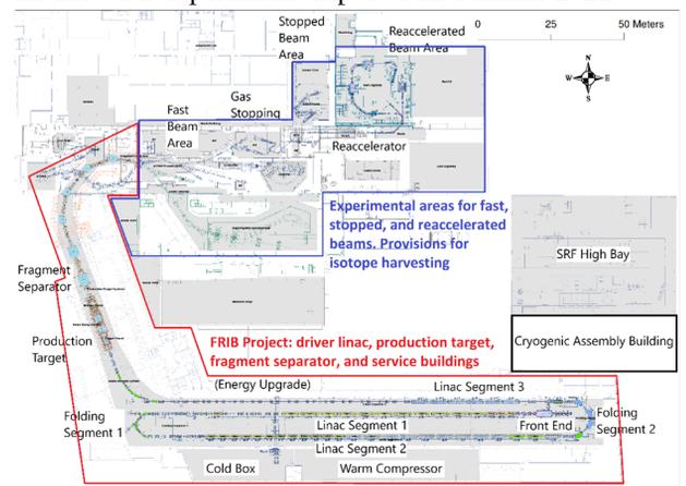
Figure 1: Layout of the FRIB linac, target, fragment separator, and experimental areas.
