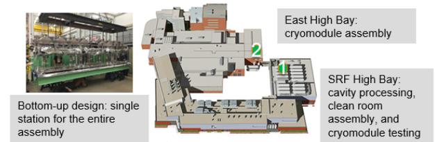
Figure 5: FRIB cryomodule production facility layout.
