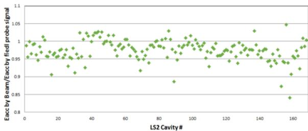
Figure 11: Comparison of  $E_{acc}$  measurements by beam and pickup antennas for LS2 cavities.
