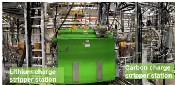
Figure 8: Liquid lithium and rotating carbon foil charge strippers installed downstream of LS1.
