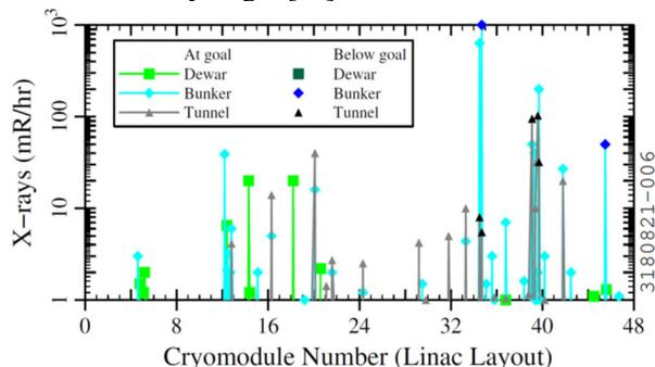
Figure 14: Cavity field emission in VTA, bunker test, and linac commissioning.
