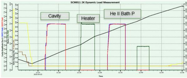
Figure 9: Dynamic load measurement for a FRIB cryomodule using  $dP/dt$  with an electrical heater.
