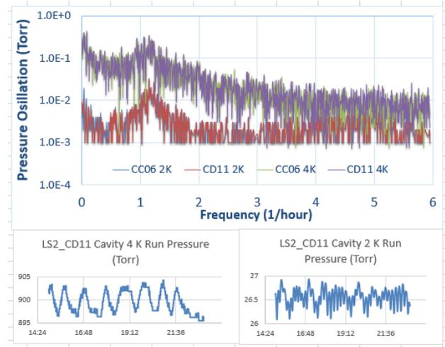
Figure 12: Bath pressure stability at 2 K and 4 K for a  $\beta = 0.29$  cryomodule (CC06) and a  $\beta = 0.53$  cryomodule (CD11) in LS2 during ARR05.
