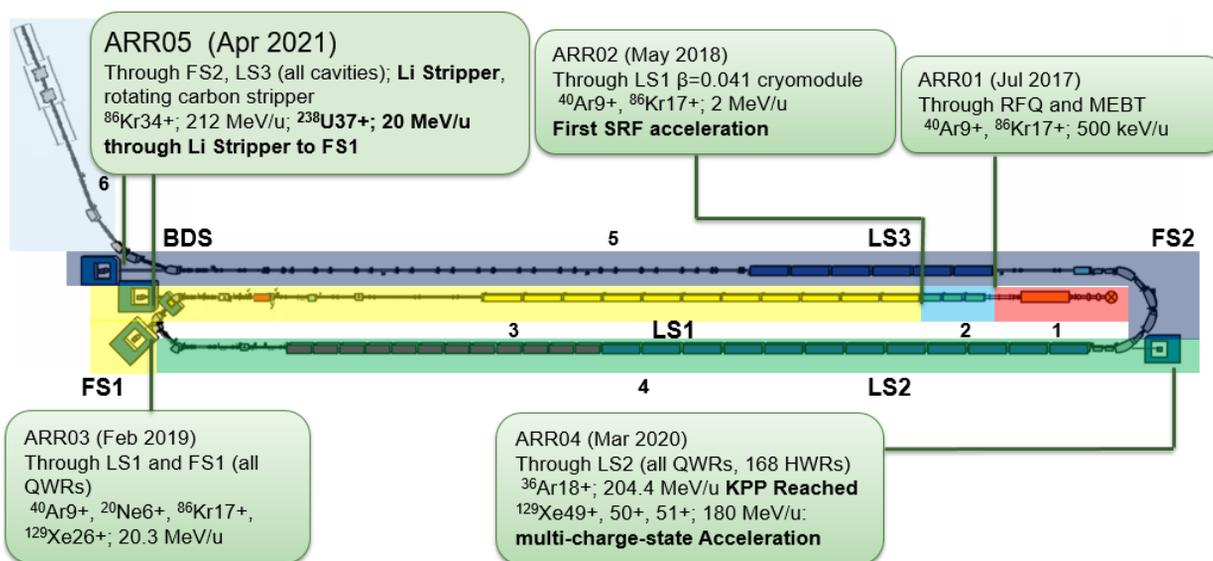
Figure 7: FRIB linac phased beam commissioning: configuration, timeline, and results.
