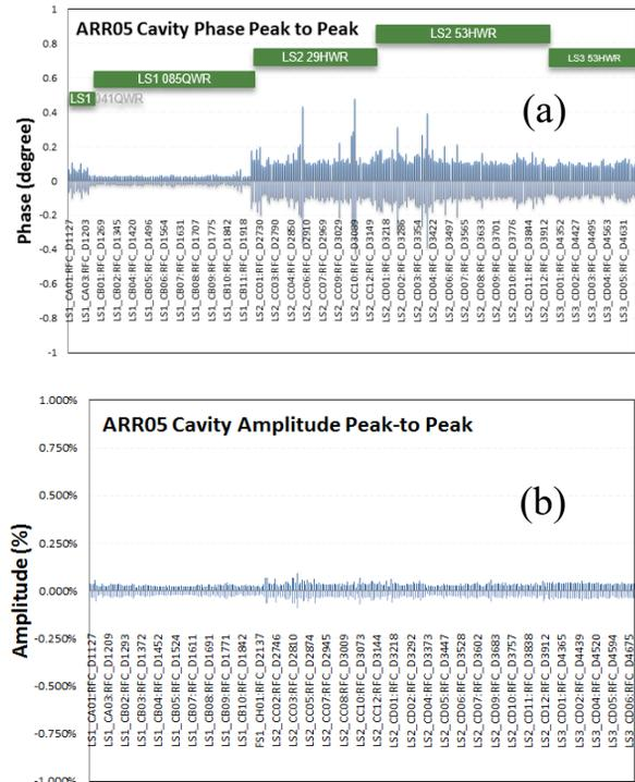
Figure 13: ARR05 cavity resonance control performance: peak-to-peak (a) phase and (b) amplitude.
