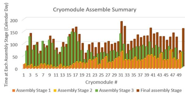
Figure 6: Times at each assembly stage for FRIB cryomodules. 1: baseplate pre-assembly ready; 2: cold mass ready to install to baseplate; 3: cryogenic system installed; 4: final assembly ready.
