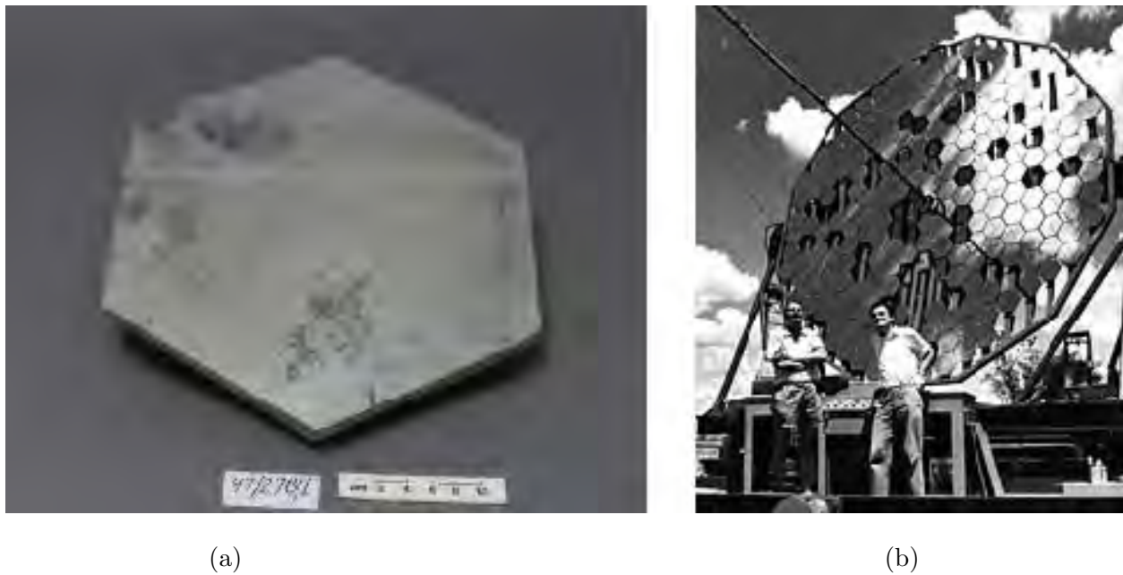
Figure 4.9: (a) A single hexagonal mirror (image: court. Sydney Powerhouse Museum) and (b) one of the reflectors of the stellar interferometer [Han74a].
