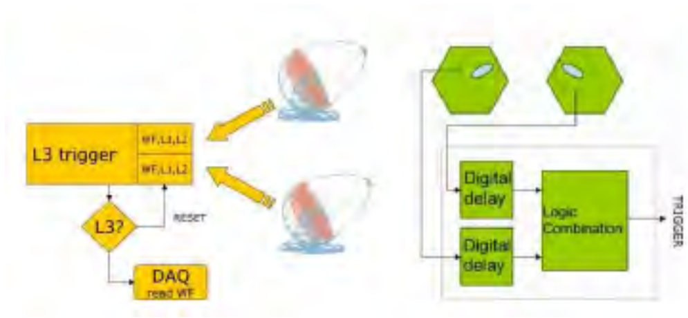
Figure 2.13: The third level trigger (L3) operative scheme.
