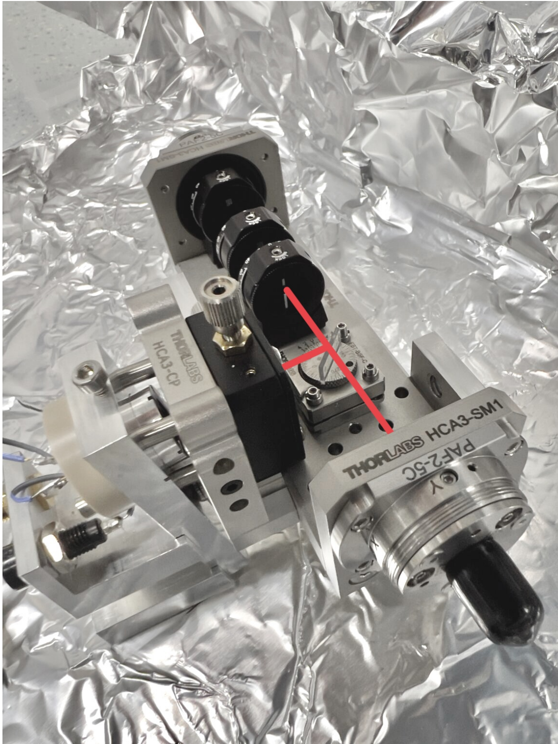
Figure 5.13: Photography of the Amplitude Stabilization scheme which includes a \lambda/4 , \lambda/2 and linear polarizer module for polarization cleaning and a FiberBench Beamsplitter Module 96:4 for amplitude stabilization and feeding with light the MZI.
