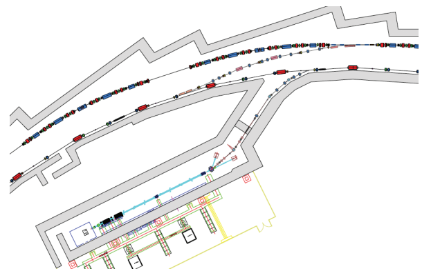
Figure 1: Layout of Sirius injection system with a 150 MeV Linac and a 3 GeV booster in the same tunnel as the storage ring.
