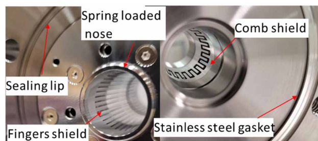
Figure 8: Pictures of the 21mm diameter RF shielding of the bellow (left) and valve (right).
