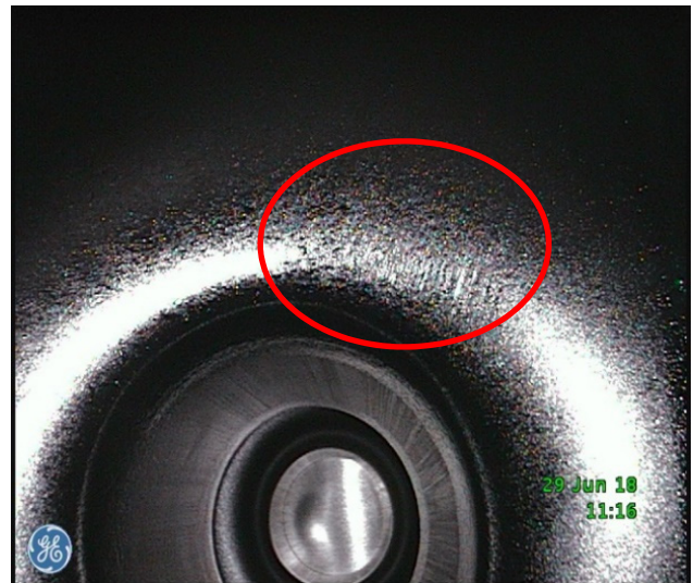
Figure 6: Surface scratches/ledges on the drift tube, possibly due to acid erosion, observed after the first Dewar test ( \beta = 0.53 HWR, S53-113).
