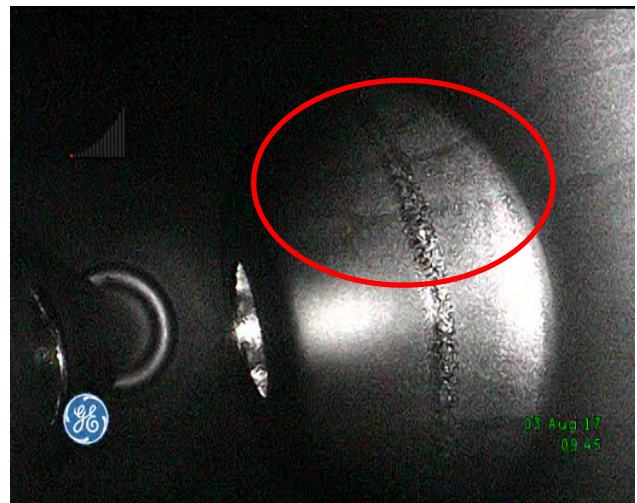
Figure 7: Acid vapour marks on outer conductor observed after first Dewar test ( \beta = 0.085 QWR, S85-951).
