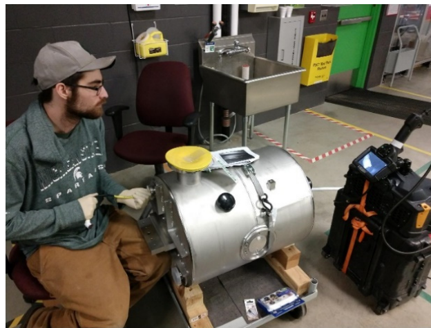
Figure 2: HWR polishing using the borescope (right) and a manual polishing tool (left).
