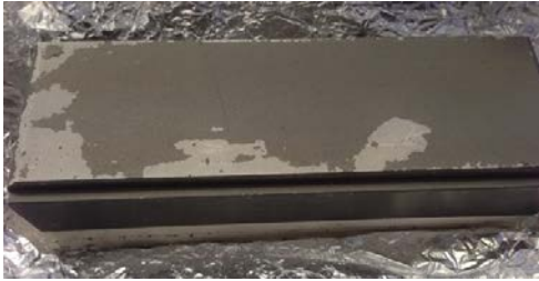
Figure 4: Coated boron nitride blocks after bake-out at 300°C.
