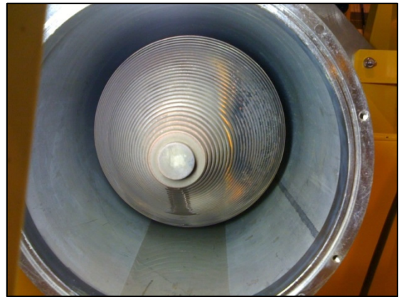
Figure 5: Klystron collector showing traces of overheating (2010).
