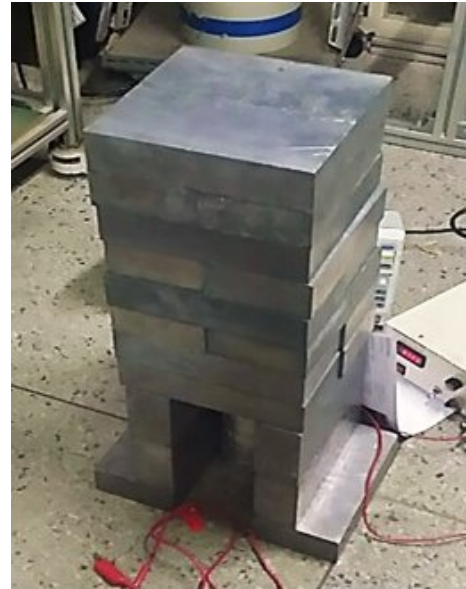
Fig. 6. (Color online) Experiment 1. Shape of the lead shield. The detector is located under the lead shield.
