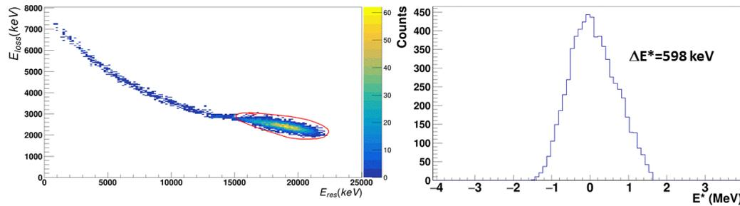
**Fig. 3:** The telescope data are shown on the left, where  $E_{loss}$  vs  $E_{res}$  represents the energy loss in the DSSSD vs total energy deposited in the thick Si layers. The red contour selects the region of elastically scattered protons, which are projected on the spectrum right to provide an indication of the excitation energy resolution. The standard deviation is indicated on the spectrum to the right.
