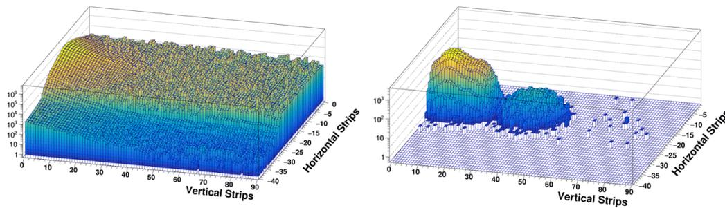
**Fig. 4:** Heavy residue position data shown without (left) and with (right) selection of scattered protons measured in the telescope detector. In the figure to the right, events related to  $\gamma$ -ray emission ( $^{208}\text{Pb}$  residues) are associated with the peak to the left, while events related to neutron emission ( $^{207}\text{Pb}$  residues) are in the peak to the right.
