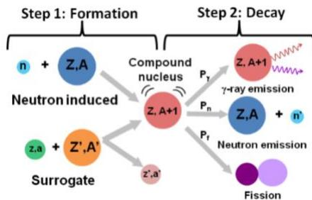
**Fig. 1:** Illustration of the two-step process, where the compound nucleus is formed in Step 1 (the formation stage) and decays in Step 2 (the decay stage) by  $\gamma$ -ray emission, neutron emission or fission. In Step 1, the same compound nucleus can be formed by either a neutron-induced reaction or through an alternative surrogate reaction which may be more experimentally feasible.
