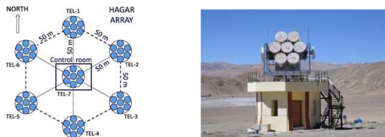
Figure 1. Schematic layout of HAGAR array (left) and one of the telescope of the array (right).
