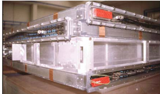
Figure 6.37: The photo of the full size prototype of the CMS DT chamber.
