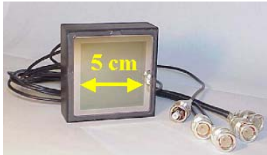
Figure 7.48: The new PLANACON TM S85001-501 hybrid photomultiplier.
