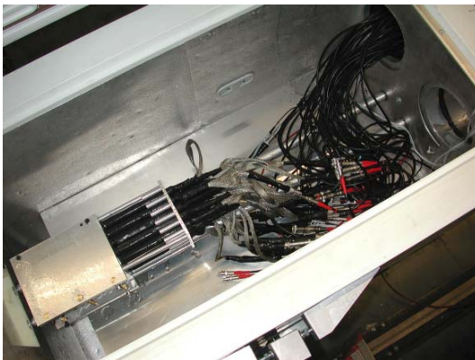
Figure 7.73: The 5×5 PWO matrix shown inside the insulated box including the photomultipliers and read-out cables.
