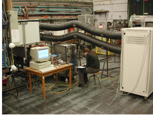
Figure 7.71: The experimental setup at the tagged photon facility comprising the cooling unit (right), the connection pipe to circulate cold dry air and the container for the test detectors (left).
