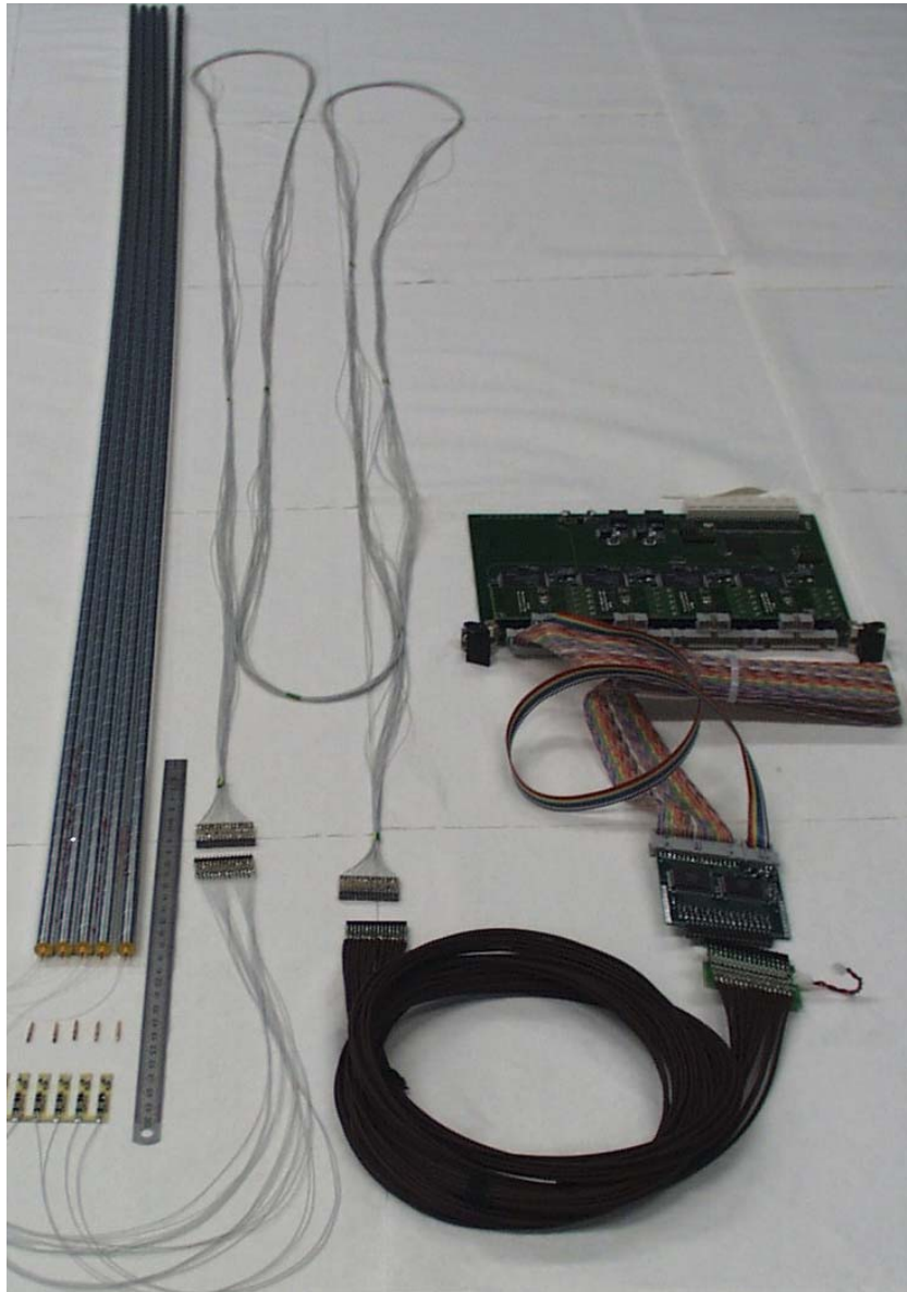
Figure 5.7: Prototype straws for the charge-division tests.
