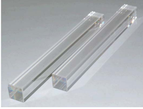
Figure 7.1: Lead tungstate crystals for \bar{\text{PANDA}} /EMC prototyping. The size of the elements amounts to 20 \times 20 \times 200 \text{ mm}^3 .
