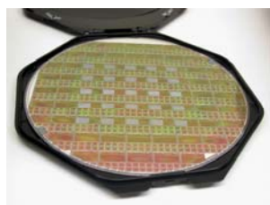
Figure 2: Sensors bonded to ROIC using DBI process
