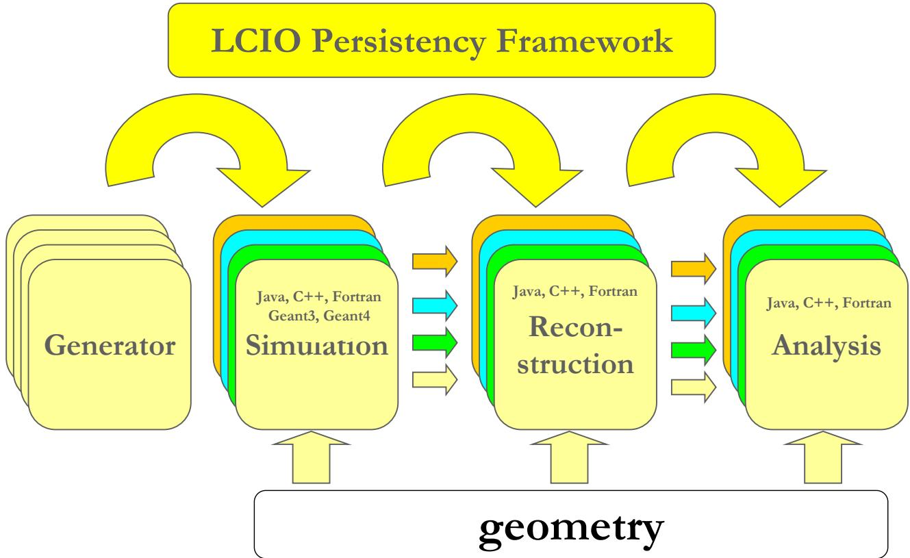
Fig. 2. Schematic showing how LCIO enables interaction between high-energy physics software written in different languages or frameworks.
