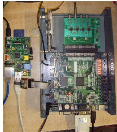
Figure 1: A view of the custom electronics used at LAGO. It consists of a daughter board with four input analog channels, a mother board based on an FPGA (Spartan 3E XC3S500K), a pressure-temperature sensor (HP3D), a GPS receiver (Oncore UT+). The main control is based on the single-board computer (Raspberry PI).
