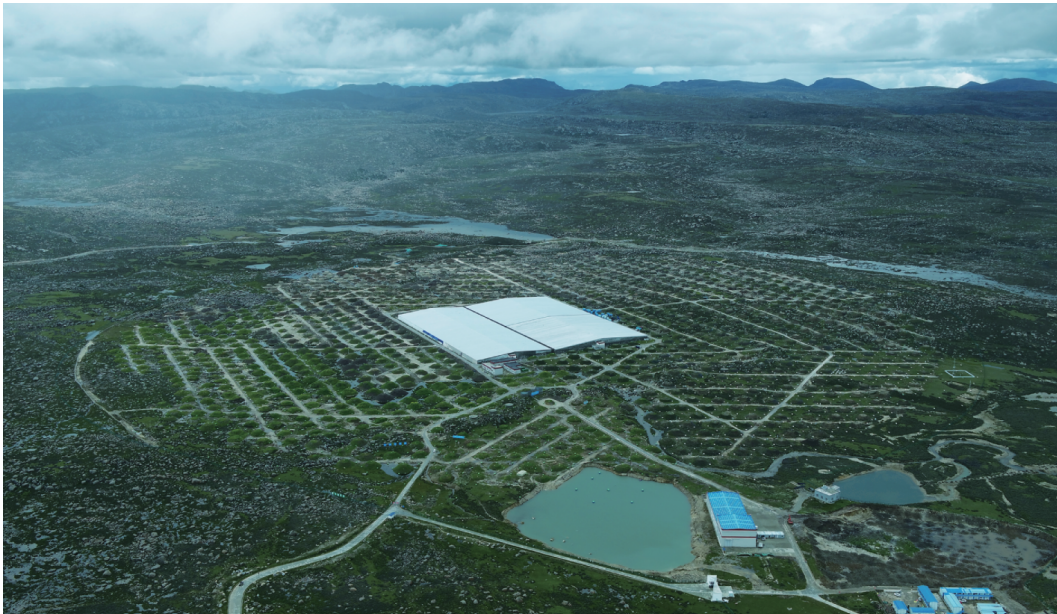
Fig. 19. (color online) Photo of LHAASO in August 2021. WCDA is the building at the center. The soil bumps are MDs. The white or green small boxes are EDs. The blue boxes beside WCDA are WFCTs.
