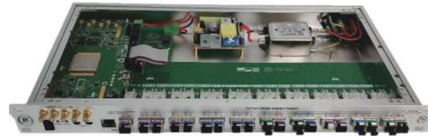
Fig. 54. (color online) Fan-less WR switch.
