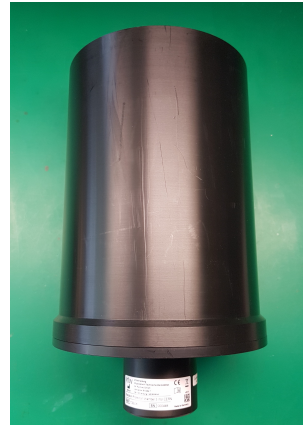
Figure 1.5: PTW PMI T32006 chamber [12]
