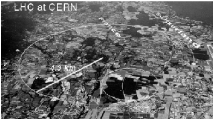
Figure 2.3: Aerial view of the LHC accelerator at CERN. The accelerator tunnel is marked in the photography. The tunnel is 100 m below ground level, and not visible from the ground. (Photography from [26]).
