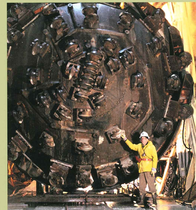
The front end of a tunnel boring machine seen at work during underground construction for the NuMI project.
