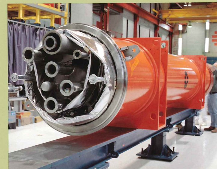
A prototype superconducting quadrupole magnet for the LHC at CERN, being assembled at Fermilab.
