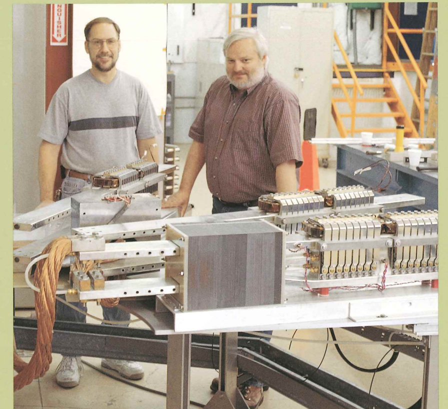
Brad Claypool (left) and Steve Hays work on power supplies for future colliders, which will have power demands of ten or more megawatts.
