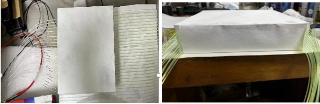
Figure 6. (1) placing the fibers in the slots of a PMMA plate beneath the container, (2) placing the fibers in the slots of a PMMA plate on the side of the container.
