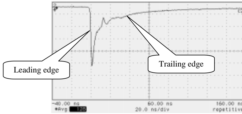
Fig.1 Current signal from a straw, filled with our Ar(65%) CO 2 (5%) CF 4 (30%) gas mixture.
