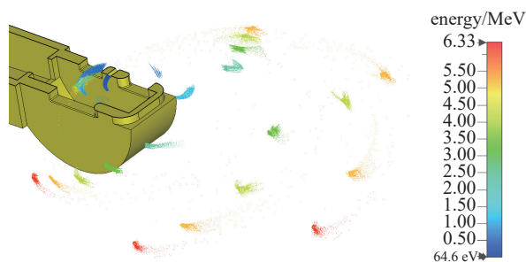
Fig. 11 3D result of electron beam dynamics in space
