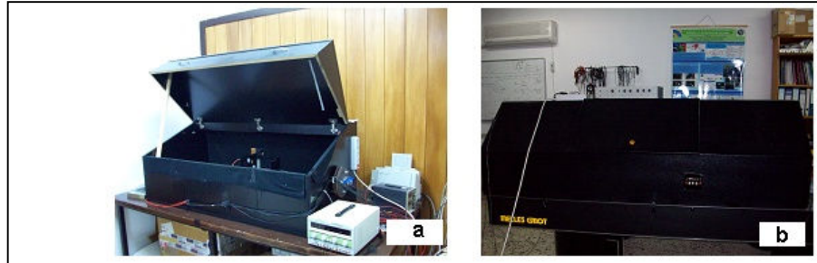
Figure 2.10. Dark boxes; a) dark, anode, linearity and collection efficiency measurements done in gain box, b) timing measurements done in timing box.
