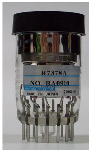
Figure 2.21. A view of the Hamamatsu R7378A PMT.
