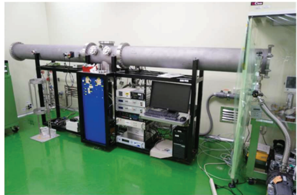
Figure 1: The sputtering system.
