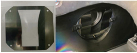
Figure 6: Design and fabrication of the coating mask and installed in the system.
