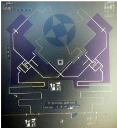
**Figure 5.** Our KID system mask design for simulation and fabrication (left) and a photograph [17] of the fabricated KID system using the hybrid fabrication process (right). The four triangular arms at the top-center are orthomode transducer based polarization antennas. From there, two 180° hybrid are seen at the left and right sides. The two snake-like structure correspond to two KIDs and the signals from them are read out by a feedline located at the bottom that runs horizontally.
