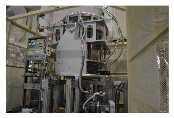
Figure 7. A picture of fully assembled GB telescope in a safety cage. A rack on the left contains service electronics to the telescope.
