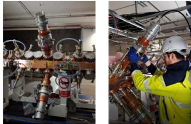
Figure 6: RFQ power couplers adjustment.
