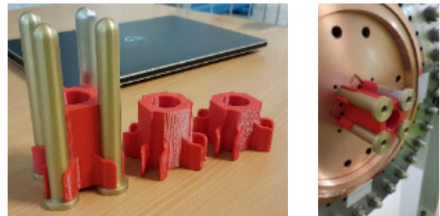
Figure 2: tunable rods on shim and inserted at one end.
